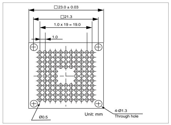
Figure 5 Recommended Dimensions for Mount Pad
